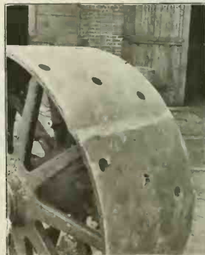
A Good Example of Welding Rolled Steel. The Rim of this Motor Truck Wheel is Formed by Rolling a Steel Plate Into Shape, Welding the Two Ends Together. The Illustration Shows it Before and After Finishing. The Metal at the Weld Was Cut Down Until It Was No Greater in Thickness Than That in the Plate and Still It Was Sufficiently Strong for this Severe Service. Finished Rim at Right.
