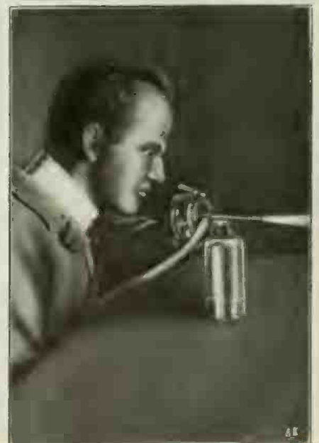
Fig. 90. Another Sodium and Water Experiment—After the Action Stops the Air Orifice of a Bunsen Burner is Held Over the Bottle, Giving a Yellow Color to the Flame.
