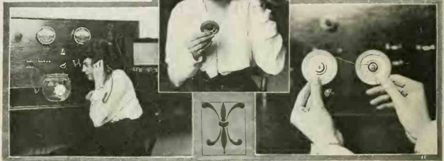
Left: Even When Submerged the New Transmitter Gave Perfect Transmission Thru Surface of Water. Center: A Casing Is Not Required for Talking. Right: Front and Rear Views of New Microphone Showing Construction Details.
