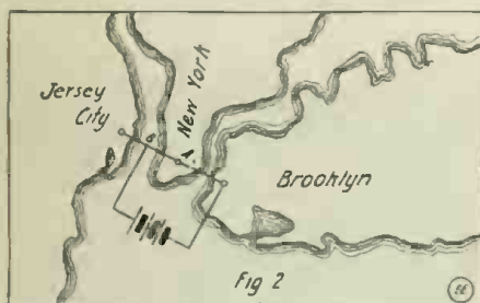
Theoretical Electric Circuit Devised by Author to Show That Changes in Resistance, Etc., of Single Conductor Extension at B Will Not Affect Current in Closed Battery Circuit.
