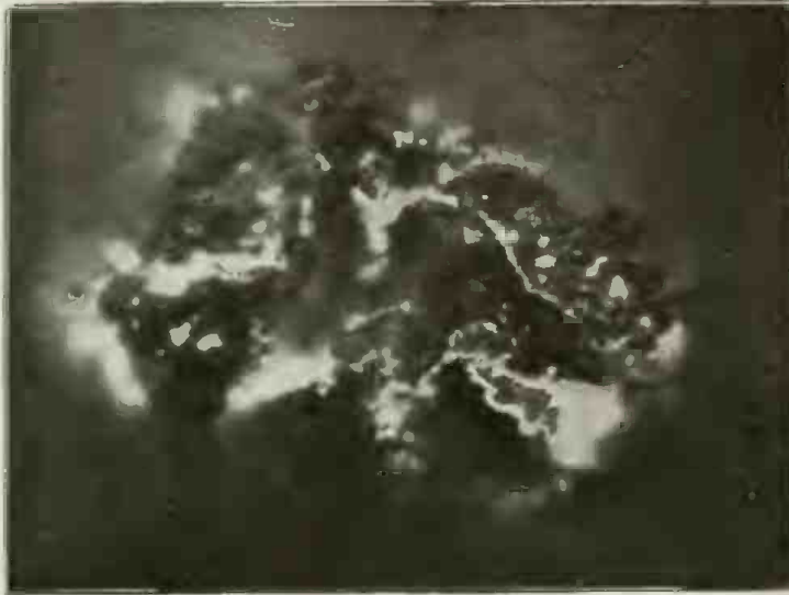
A Piece of Pitchblende from St. Joachimsthal Photographed By Its Own Rays. The Pitchblende Was Spread Evenly Over Black, Opaque Paper Covering the Photographic Plate.
