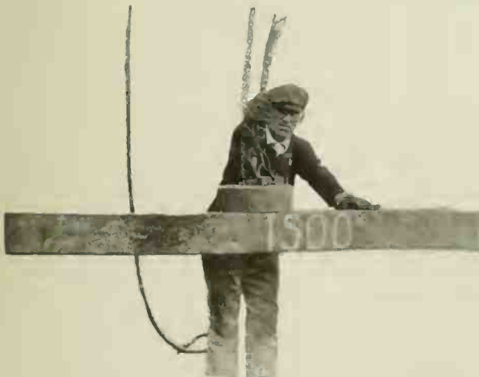
Here We Have the "Man With the Magnet," Who Is Almost as Famous Nowadays as the Immortal "Man With the Hoe." The 12-inch Electro-Magnet Is Shown Lifting a 1,500-lb. Steel Billet.
