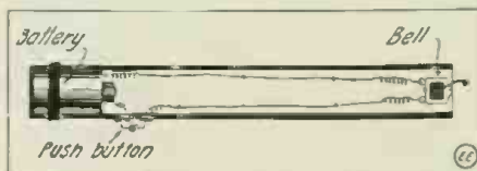
Instead of Taking Chances With the Old Spool Window Ticker on Halloween, Use This Simple Electric One on a Long Pole.
