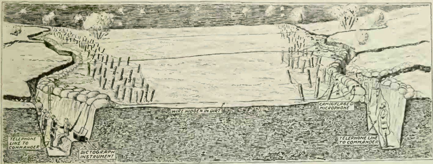
Listening to the Doings in the Enemy's Trenches By Means of Supersensitive Microphones is a Recent Idea. It Shows a New Way How to Get Advance Information, as, for Instance, Just When the Enemy Intends to Attack, Etc., Etc.
