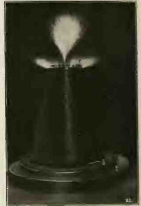
Fig. 1. Illustrating the Vigorous High Frequency Discharge From Free Electrode, As Well As Top, of Oudin Coil of Good Design.
