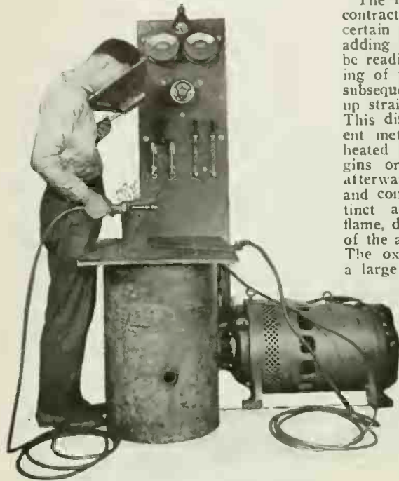
Complete Electric Arc Welding Outfit. It May Be Moved From Job to Job When Desired. Note the Glass Shield Which Operative Uses to Protect Eyes From Blinding Glare.
